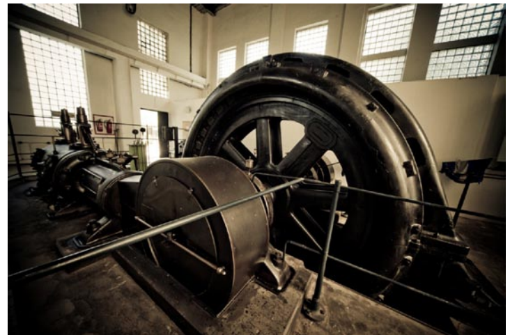
An electrical reciprocating compressor – A Czech national treasure
